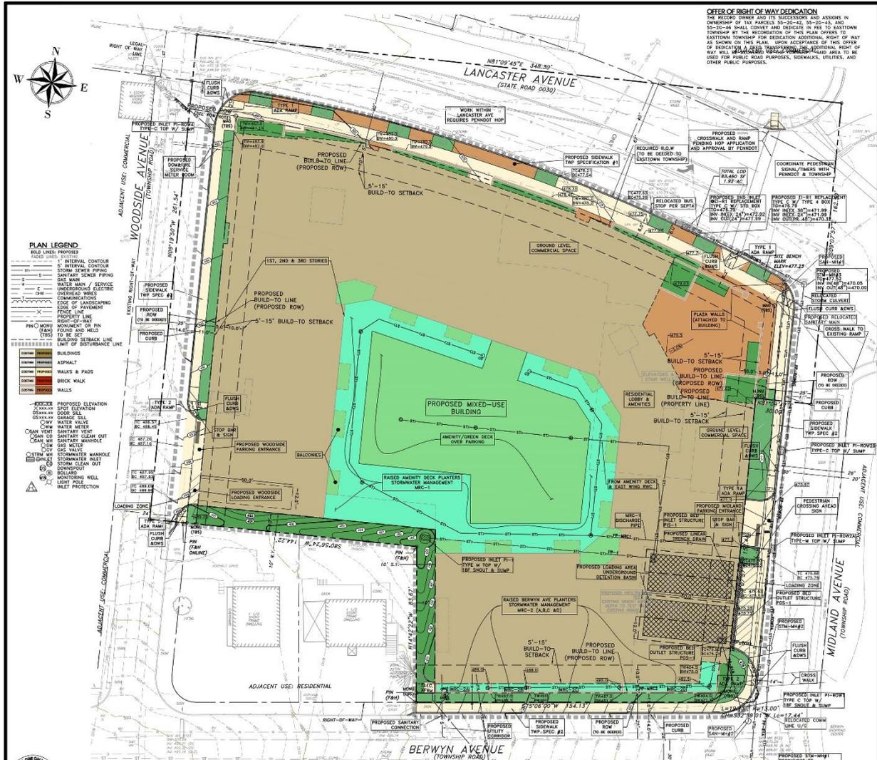
Site Plan Detail, Sheet 5: Land Development Plan, Post-Construction Stormwater Plan
